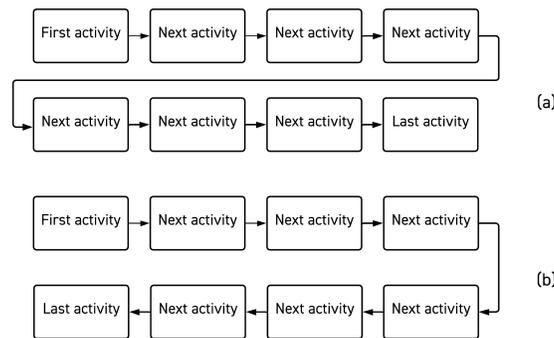
Figure B-1 (a) Recommended way to fold a horizontal flow, (b) not recommended
