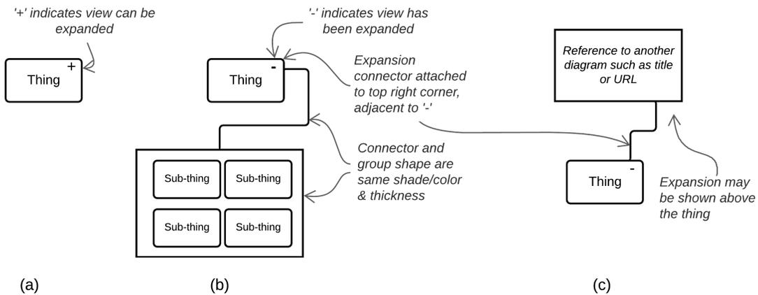
Figure 6-3 Expanded and contracted views
